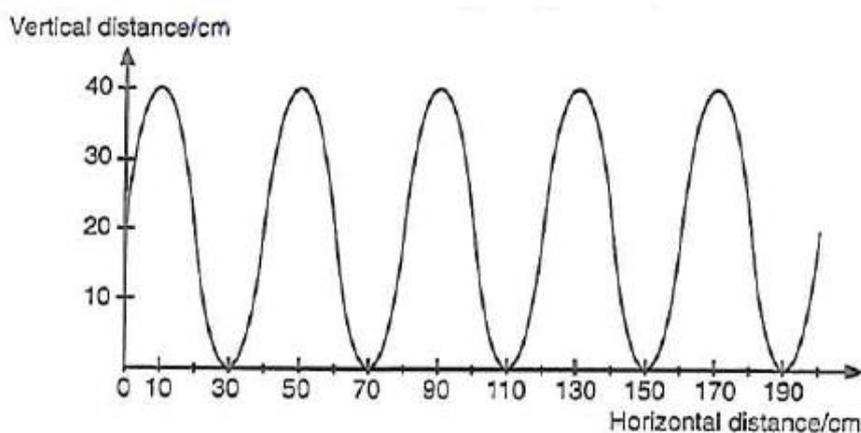
3 A vertical vibrator generates waves on a string. It takes 0.25 s to produce a complete wave of wavelength 0.80 m on the string.
