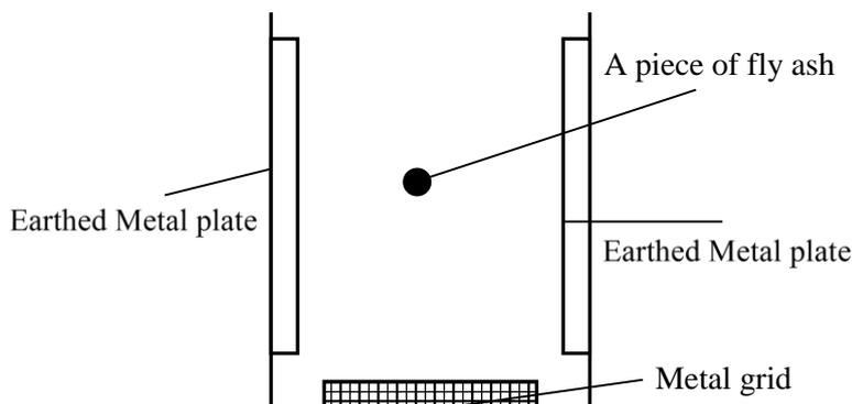
5 The figure shows the apparatus used to demonstrate the electric field pattern in school laboratories. Sketch the electric field patterns observed for the following electrodes.
