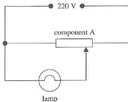
A simplified circuit diagram of the brightness control knob is shown.
