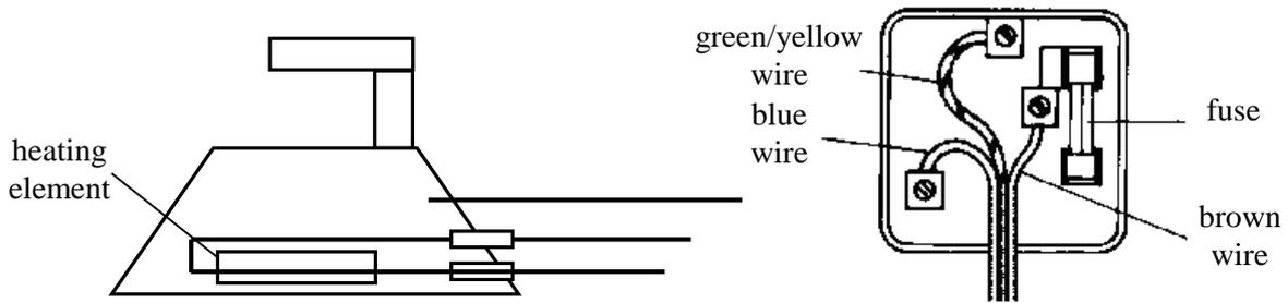
The diagram on the left shows an iron and the diagram on the right shows a three pin plug that connects the iron to the household mains. When the iron is switched on, the time taken for the iron to heat up is 1 minute. The iron is rated 1.5 kW 240 V.
